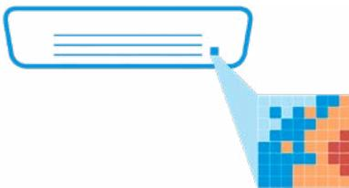
The grid eye sensor measures the surface temperature of a room by dividing it into a grid with 64 different squares.
