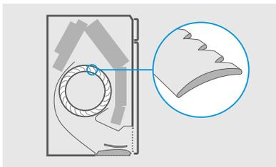
Sound dispersion and noise reduction are the results of new fan design.
